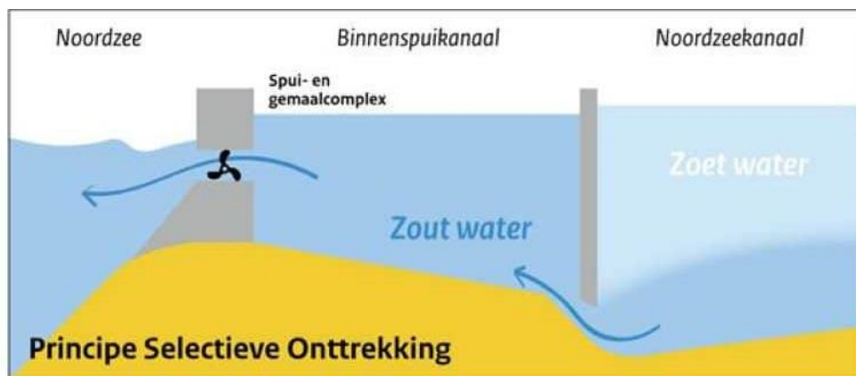
Figure 7: Diagram of the IJmuiden salt dam (right pillar). The salt dam blocks freshwater and ensures that only heavy saltwater that enters the North Sea Canal is pumped back into the North Sea [16] .
